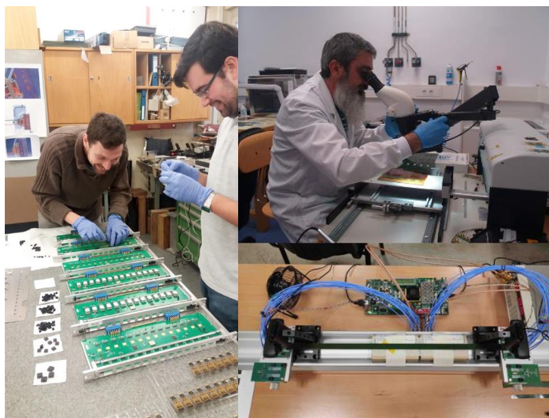
Figure 2. Assembly of Optical Power Boards, production of High Voltage cables, High-Speed data links
