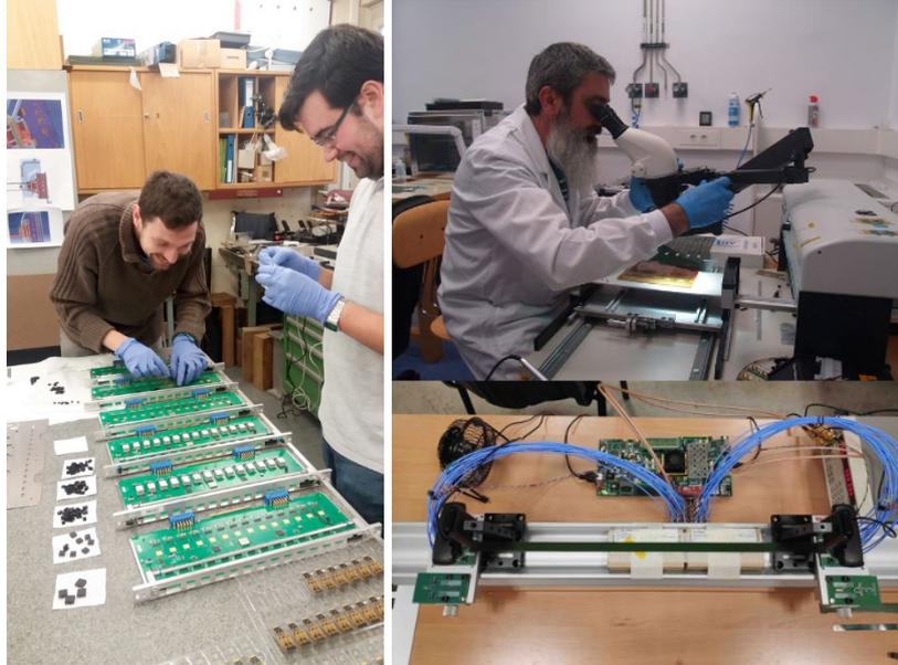
Figure 9. Assembly of Optical Power Boards, production of High Voltage cables, High-Speed data links
