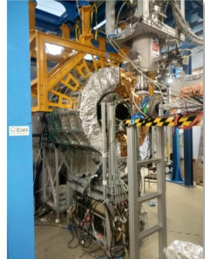
Figure 19. View of the CALIFA calorimeter installed at the nominal target position in the R3B Cave. Beam direction from right to left.
