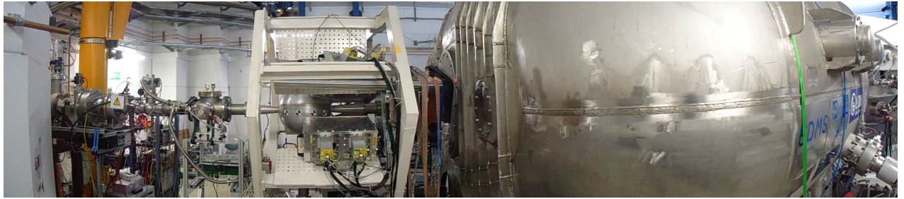
Fig.12: View of the R3B experiment in Cave C (FAIR Phase 0). From left to right we distinguish the incoming detectors, the target area with the CALIFA demonstrator installed and the Large Acceptance magnet GLAD.
