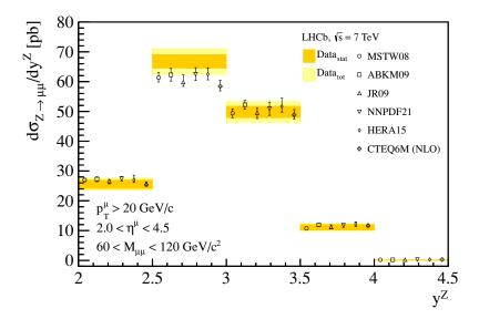
Figure 7. Differential cross-section for  $Z \to \mu\mu$  as a function of  $y^Z$ . The dark shaded (orange) bands correspond to the statistical uncertainties, the light hatched (yellow) band to the statistical and systematic uncertainties added in quadrature. Superimposed are NNLO (NLO) predictions with different parametrisations for the PDF as points with error bars; they are displaced horizontally for presentation.
