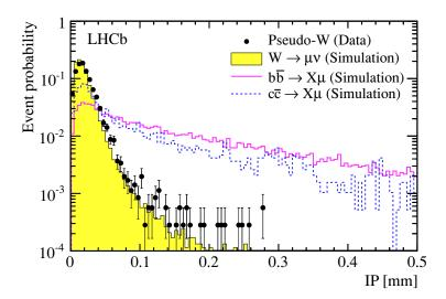
**Figure 3.** Muon IP distribution for pseudo-W events as points, W-MC as a yellow (shaded) histogram, and muons from simulated semi-leptonic decays of hadrons containing a b quark in the full open histogram or a c quark in the dashed open histogram. All distributions are normalised to unity.
