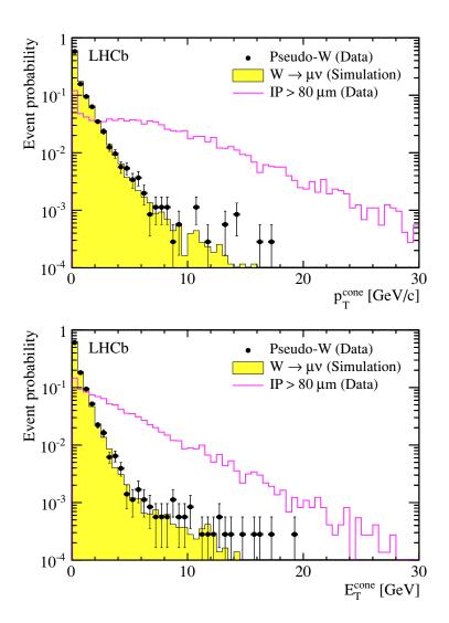
**Figure 2.** Distributions for  $p_{\rm T}^{\rm cone}$  (top) and  $E_{\rm T}^{\rm cone}$  (bottom). The points are for muons from pseudo-W data, the yellow (shaded) histograms are for W-MC simulation, while the open histograms are for muons from QCD background with IP > 80  $\mu$ m from data. All distributions are normalised to unity.
