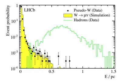
**Figure 4.** E/pc for pseudo-W events as points, W-MC as a yellow (shaded) histogram, and for hadrons from randomly triggered events in the open histogram. The energy E is the sum of the energies in the electromagnetic and hadronic calorimeter associated with the particle. All distributions are normalised to unity.
