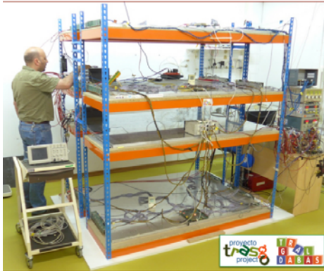
Figure 4. Picture of the TRAGALDABAS Detector System based on four planes of Resistive Plate Chamber detectors
