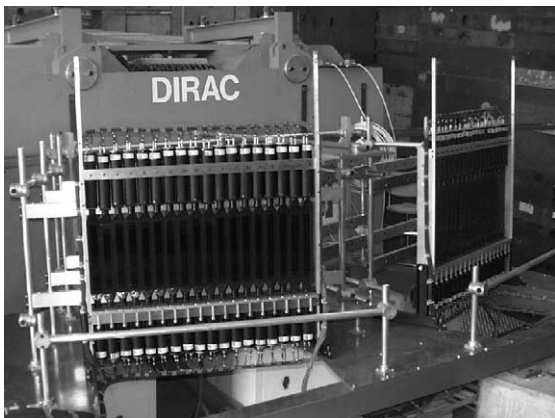
Fig. 3. Photography of the TOF detector during installation in the DIRAC experimental area after the dipole magnet.
