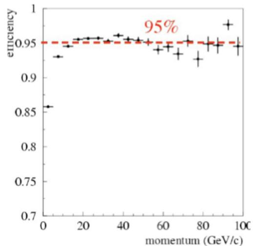
**Figure 3.** Efficiency of track reconstruction versus momentum.
