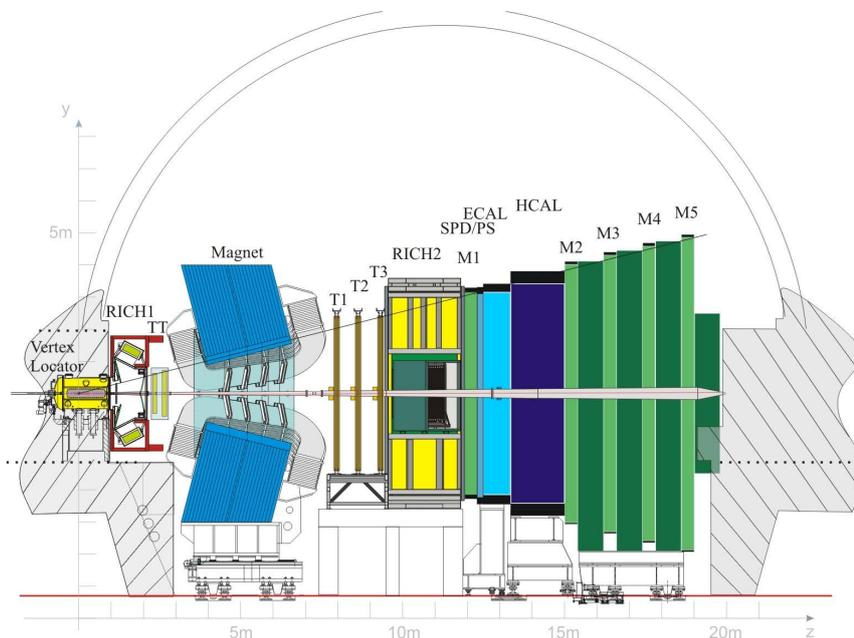
**Figure 1.** Side view of the *LHCb* detector. The interaction point is at the left. The following components are indicated: the Vertex Locator (VELO), the dipole magnet, the two RICH detectors, the four tracking stations TT and T1-T3, the Scintillating Pad Detector (SPD), Preshower (PS), Electromagnetic (ECAL) and Hadronic (HCAL) calorimeters, and the five muon stations M1-M5.
