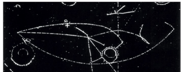
The neutrino interaction \nu_\mu from the left produces 3 charged particles, all of them identified as hadrons , since they interact with nuclei in the liquid filling the chamber. It is thus excluded that any of them can be a muon ( source: CERN ).
