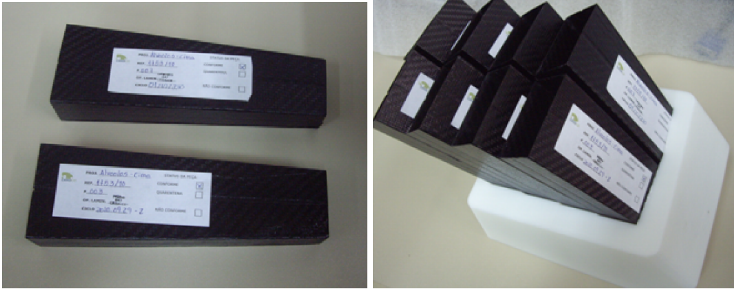
Figure 6.2.: Hand-made epoxy-carbon fibre alveoli, 0.25 mm thick walls, for the preliminary tests.
