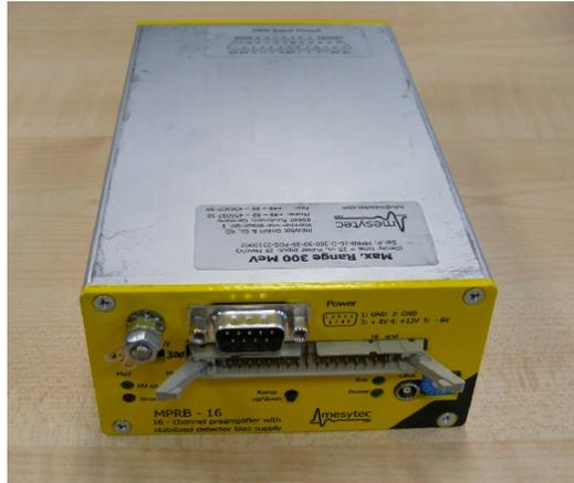
Figure 4.5: Mesytec MPRB-16 pre-amplifier front panel
