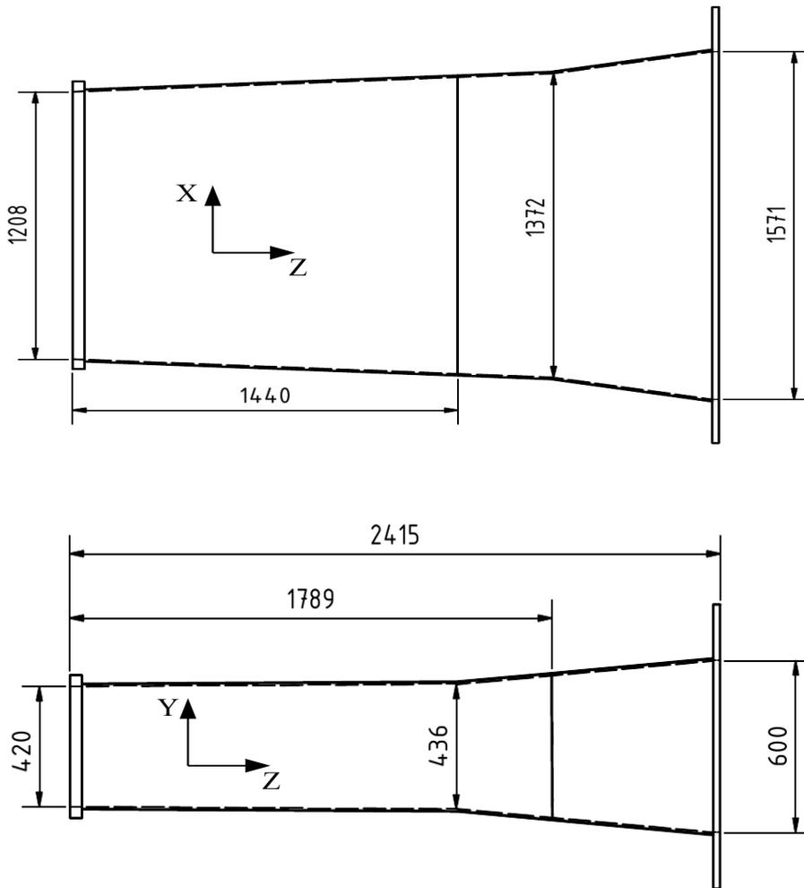
Figure 2.11: Dimensions of the gap in ALADIN dipole, all in mm.
