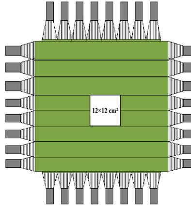
(a) Detector for light charged particles.
