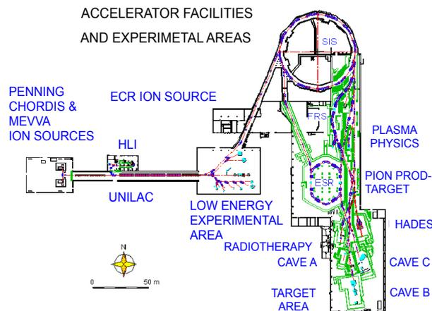
**Figure 2.1:** The GSI (Darmstadt) experimental facilities. In this drawing we can observe the two acceleration stages, the UNILAC and SIS, and the experimental areas, in particular the Fragment Separator (FRS) and Cave C.
