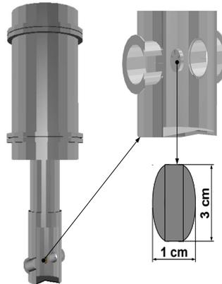
*Figure 2.5:  $H_2$  target.*
