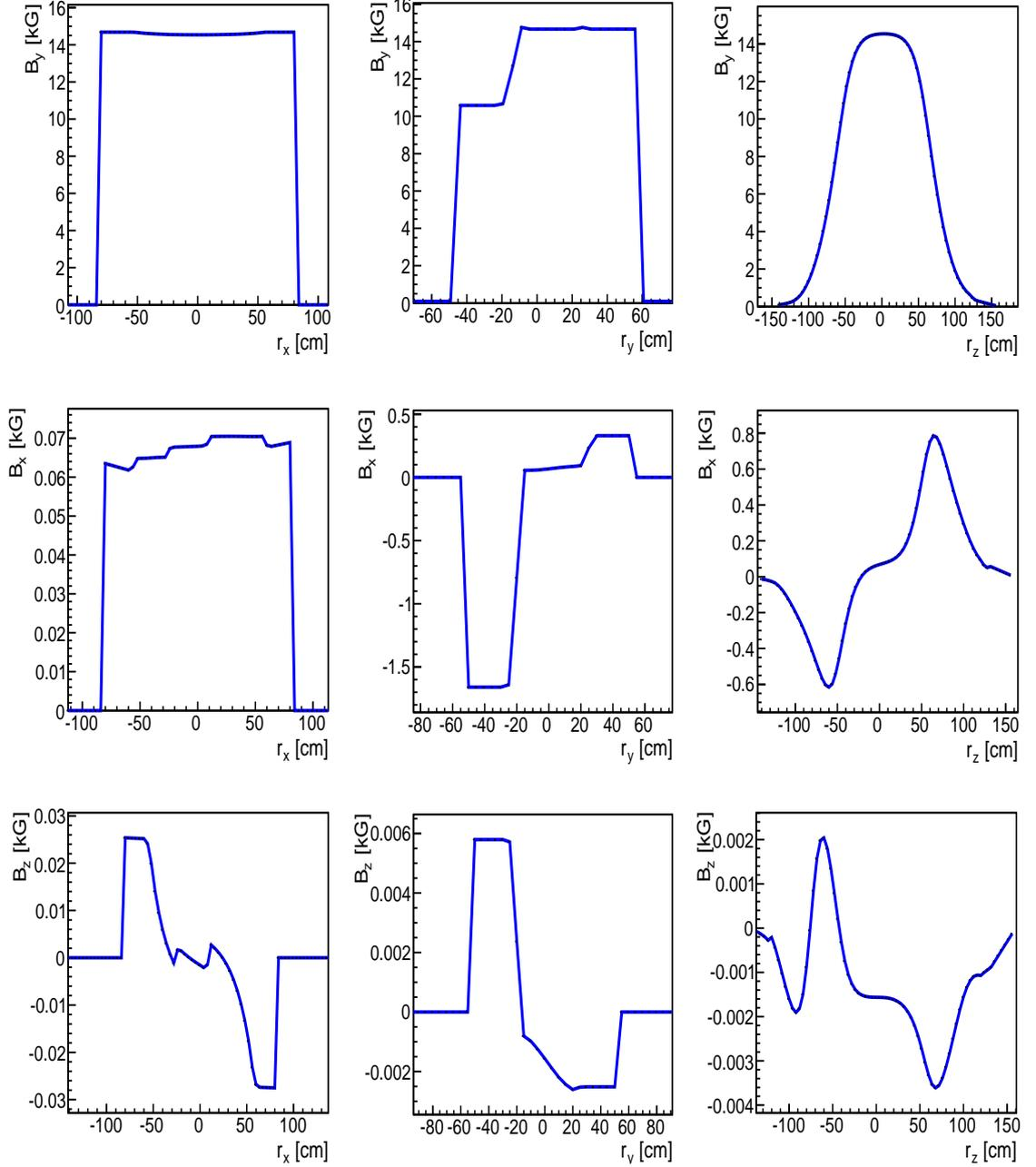
**Figure 2.12:** The Aladin magnetic field component in the  $B_x$ ,  $B_y$  and  $B_z$  direction as a function of the  $r_x$ ,  $r_y$  and  $r_z$  direction (see figure 2.4). In the graph  $B_y$  vs.  $r_y$  we observe that the magnetic field is not symmetric but it is not important because the  $y$  dimension of Aladin is  $[-21, 21]$  cm.
