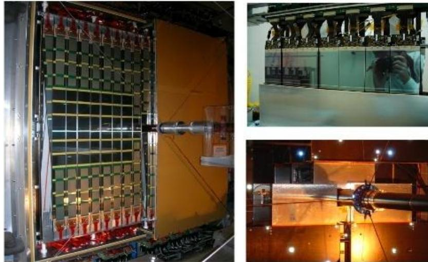
Figure 2.8: View of the TT installed in LHCb (left) with one boxes open and the sensors inside. View of the first IT station (bottom right), and detail of one of the detector boxes in semi-open position (top right).
