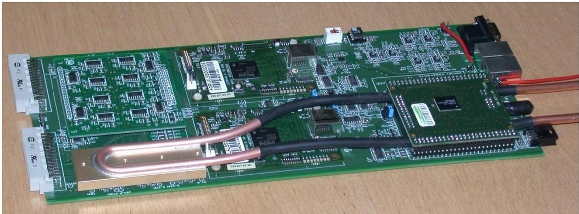
Figure 3.8: Final Control Board with the final water cooled cooling block.
