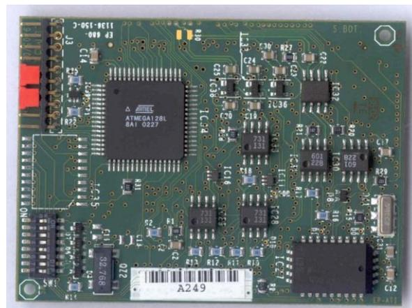
Figure 8.19: ELMB plug-in board.
