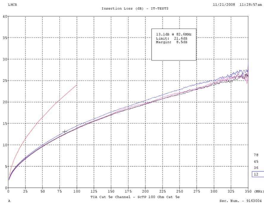
Figure 12.28: Sample results of the SPECS Ethernet cables. All of them were even within the CAT5e specifications. The figure in the right is a zoom of that in the left.
