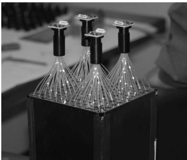
Figure 3.63: Prototype EMCal module. The back enclosing structure is removed so that the converging, wavelength shifting fibres are visible from each of the 4 towers. The charge sensitive preamps are shown integrated directly to the APD (not visible).
