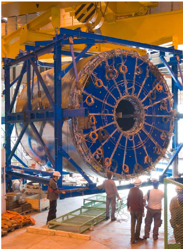
Figure 3.37: The TPC as assembled above ground on its way to the ALICE cavern.
