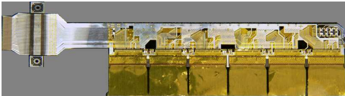
Figure 3.27: Photograph of a hybrid. Each hybrid was tested individually, using the connection area at the left side of the flex. This part was cut off before connecting to the sensor. The lower part of the photograph shows the six chip-cables which will connect the HAL25 chips to the sensor. The chips themselves are covered by the chip-cables and not visible in this picture. The aluminium clamps connecting to the cooling tubes are on the reverse side of the hybrid.
