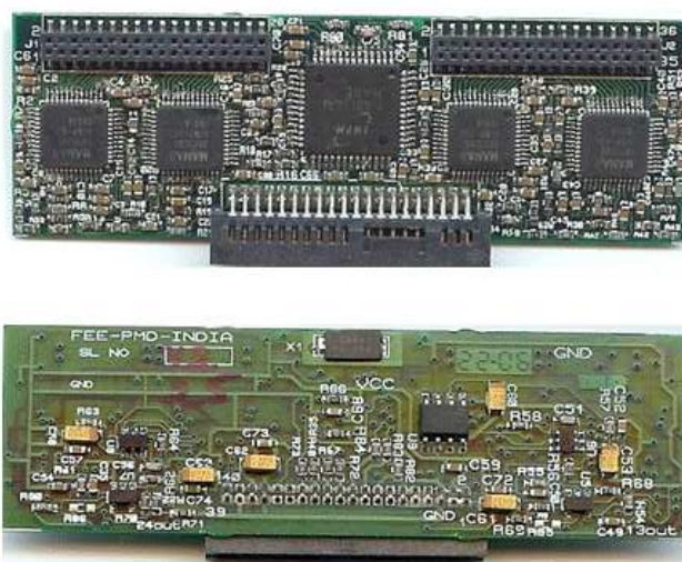
Figure 5.10: Photograph showing both sides of the Front-End Electronics board of the PMD. Four MANAS chips along with the MARC are clearly seen.
