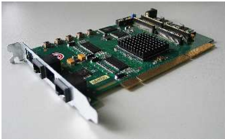
Figure 6.8: H-RORC data pump and FPGA coprocessor.
