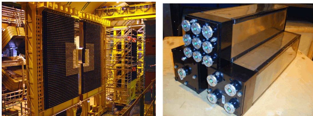
Figure 6.25: Downstream view of the ECAL installed (but not completely closed) with the exception of some detector elements above the beam line. Outer, middle and inner type ECAL modules (right).
