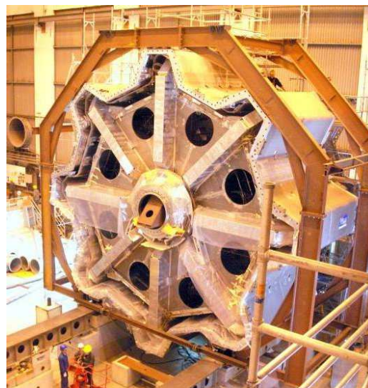
Figure 2.5: End-cap toroid cold mass inserted into the cryostat. The eight flat, square coil units and eight keystone wedges (with the circular holes) are visible.
