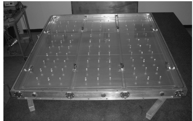
Fig. 3. The three radiator vessels equipping one HMPID module.
