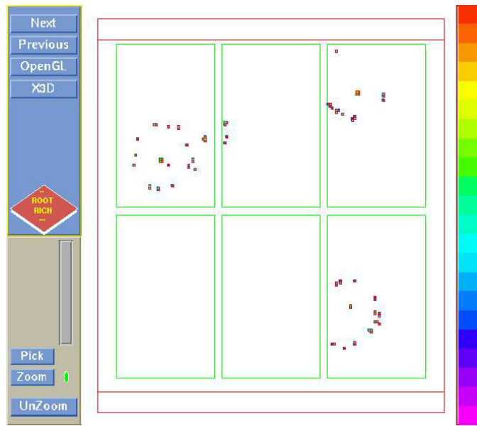
Figure 4.11. AliRoot event display of HMPID response. The rectangles correspond to pads with signals over threshold (digits).
