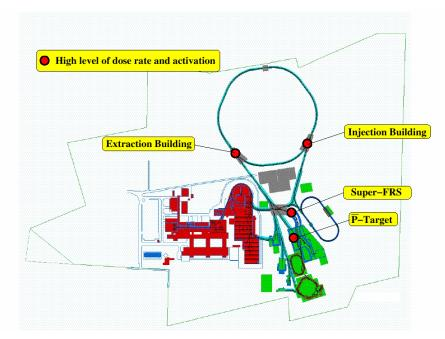
Figure 1.2: Overview of the new facility and position of the sites exposed to high neutron flux.
