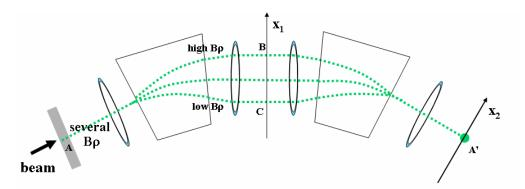
Figure 2.2: Schematic functioning of the FRS in achromatic mode. Inserting some slits at the midplane, one can stop particles with specific magnetic rigidities and let pass only those with a selected magnetic rigidity.
