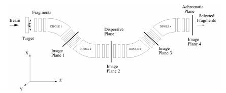
Figure 2.1: Schematic drawing of the FRS according to its ion-optic characteristics. Quadrupoles are placed before and after each dipole to define the ion-optic conditions at each image plane. In the middle (dispersive plane), there is an energy degrader.
