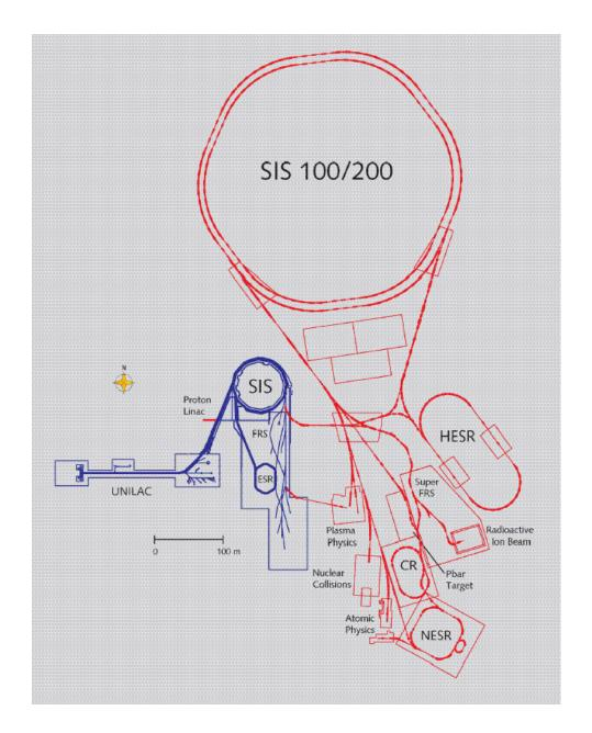
Figure 1.1: Present layout of the existing UNILAC/SIS18/ESR facility (blue) and the planned new facilities (red): the Super-conducting Synchrotrons SIS100/200, the Collector Ring CR, the New Experimental Storage Ring NESR, the Super-conducting Fragment Separator Super-FRS, the proton linac, and the High-Energy Storage Ring HESR. The drawing also shows the planned experimental areas for plasma physics, nuclear collisions, rare ion beams, and atomic physics.
