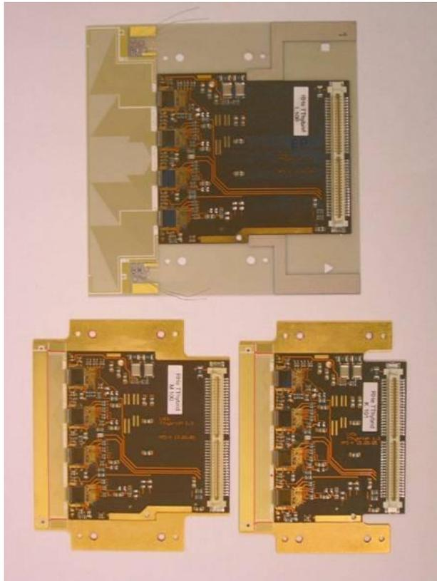
Figure 2.7: TT hybrid, flexible PCBs and pitch adapters.
