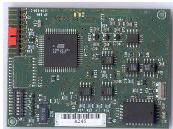
Figure 8.19: ELMB plug-in board.
