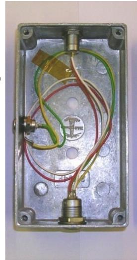
Figure 5.10: Interlock box, HV patch panel and HV modules electrical wiring to the DSS.
