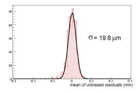
Figure 4: Offset of each ladder in IT taken from the mean of the unbiased residual distributions. The unbiased residual distributions are obtained from an independent sample of the TED data. The width of this distribution (20  $\mu$ m) is a measure for the alignment precision.
