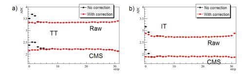
Figure 2: Raw noise and common-mode-subtracted (CMS) noise in the 32 data channels of a port for TT (a) and IT (b). It shows the effect of the header correction on the noise in the first few data channels.
