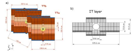
Figure 1: Layout of the full TT detector (a) and a single IT layer (b).
