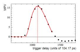
Figure 3: Pulse shape for a set of short IT ladders from the TED data. The most probable value (MPV) for each trigger delay is obtained from a fit to the S/N distribution. The overlaid curve is from a fit to a function [6] that is expected from the output of the Beetle chip.
