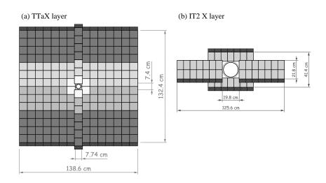
Figure 1: Layout of (a) the x layer in TTa and (b) a x layer in IT station 2.
