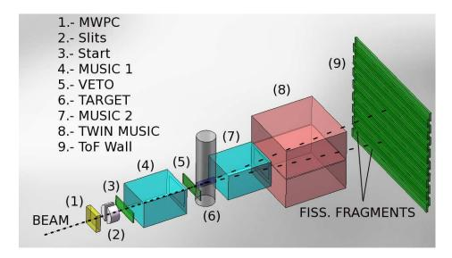
Figure 3.1: Schematic drawing of the experimental setup used in the present experiment.
