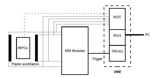
Figure 4.17: Scheme of the fADC-based data acquisition system.
