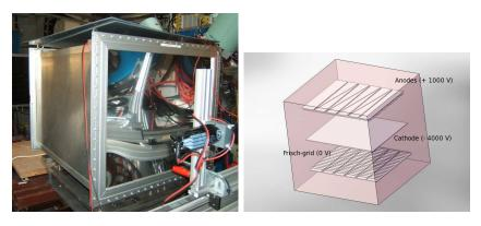
Figure 3.2: Picture of the Twin MUSIC detector and schematic representation of the two active volumes with the central cathode and the anodes.
