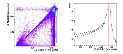
Figure 3.4: Left panel: Scatter plot of the amplitudes of the signals registered with the two MUSIC detectors. The rectangular selection represents the region were fission residues were expected. Right panel: Energy Loss signals provided by the MUSIC 1. The region between the red lines corresponds to <sup>208</sup>Pb beam particles.
