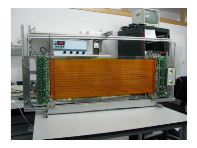
Figure 4.40: Multi-strip single-gap tRPC module for the iToF.
