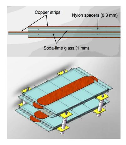
Figure 4.8: Upper panel: Lateral view of the schematic representation of a small double gas-gap prototype. Lower panel: Top view of two double gas-gap prototypes with a single strip (RPC-11).
