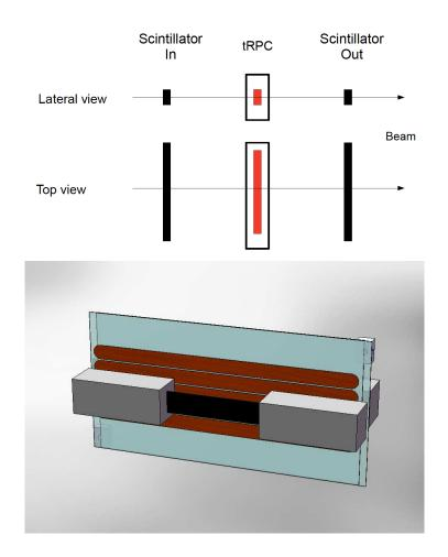
Figure 4.16: Upper panel: Scheme of the scintillator-based external trigger for efficiency and timing measurements. Lower panel: Layout of the tRPC placed in between two scintillation detectors.
