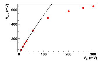
Figure 4.12: BFR92A+OPA657 FEE amplitude calibration curve (See text for details).
