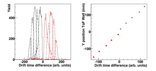
Figure 3.9: Left panel: Difference of the drift times measured in the first and fourth anode of both parts of the Twin MUSIC in coincidence with each cell. Right panel: Calibration of vertical position of the boundaries of the different cells as a function of the drift time. Red squares and blue circles refer to the lower and the upper part of the Twin MUSIC, respectively.
