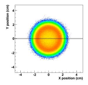
Figure 2.6: Simulated fission fragments spatial distribution in the double plastic scintillator plane for the reaction  $^{181}$  Ta+p at 1 A GeV. The area between both solid lines represents the size of the gap.
