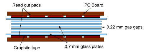
Figure 4.7: Schematic drawing of a multi-gap tRPC.
