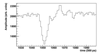
Figure 4.18: Typical pulse registered with fADC data acquisition system. The pulse corresponds to a  $^{136}Xe$  ion detected in the RPC-30 prototype. Each channel in the y and x axis corresponds to 0.5 mV and 500 ps, respectively.
