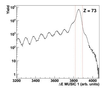
Figure 2.7: Energy loss signals provided by the MUSIC 1. The region between the dotted red lines corresponds to  $^{181}$  Ta.
