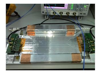
Figure 4.10: Two identical RPC structures shown in Fig. 4.9 assembled in an aluminum support (RPC-30).
