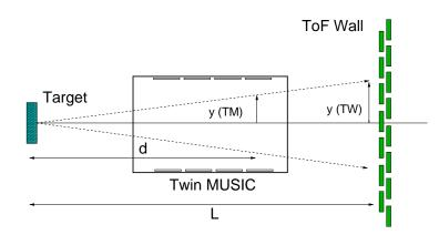
Figure 3.8: Determination of the vertical positions in the ToF Wall and in the fourth anode of the Twin MUSIC.
