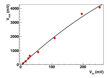
Figure 4.14: BFR92A+MAXIM-4224FEE amplitude calibration curve (See text for details).
