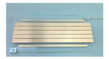
Figure 4.9: Single-gap self-contained multi-strip tRPC (RPC-30). The gas mixture is supplied via both rectangular aluminum pieces.
