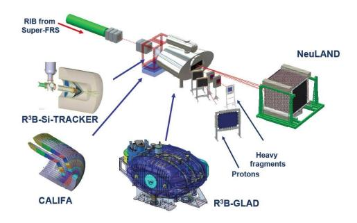
Figure 4.2: Conceptual drawing of the  $R^3B$  experimental setup. Figure taken from [R3B].
