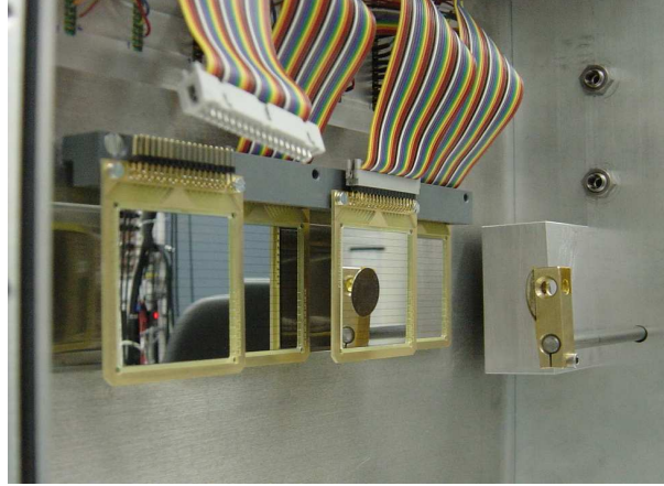
Figure 4.2: Picture of the stack of 4 DSSD mounted into the vacuum chamber
