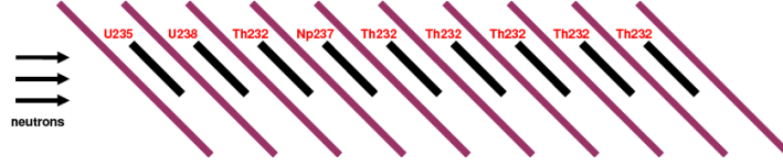
Figure 3.3: Top view of the experimental setup with ten PPAC detectors and nine targets in between. All the elements are tilted 45^\circ around the vertical axis to cover a broader angular range. Targets are labelled from 0 to 9 following the neutron beam direction.
